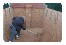
Note how the wet top soil sticks to the bed. Hundreds of pounds of material can get stuck. Scraping beds is unproductive as well as dangerous work, and scraping with heavy equipment can damage the bed. With Matrox®/ Ramex® liners, you never need to scrape a bed.
