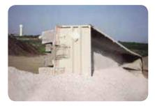
Matrox®/Ramex® liners reduce dump angles by as much as 40%. Lower dump stages reduce the chances of rollover accidents due to load hangup and reduce the chances of equipment striking overhead obstructions such as power lines or trees.
