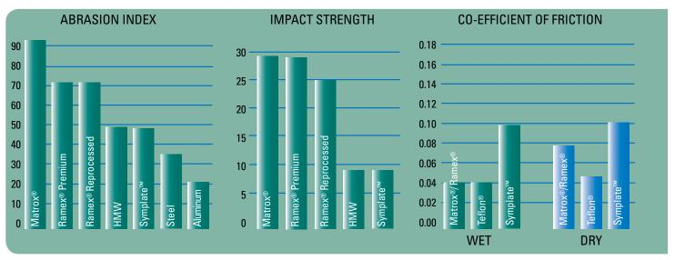
The Abrasion Index measures the amount of material retained after an extended period of wear.
